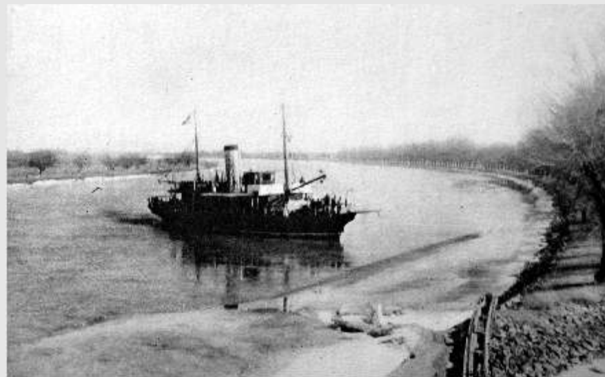
Concordia Hydrographic ship (Built in 1924, 340 PH, 31.50 m length, 7.30 m breadth, 3.50 m draught, 250.99 t brute tone, 9.6 running-knot speed)
